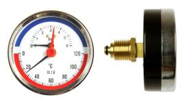
Good value combined instrument for pressure and temperature measuring. The gauges have an automatic closing valve that makes it possible to exchange the combined pressure and temperature gauge without emtying the heating system.
