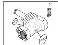
3. The arrow cast on the body and cover must point in the direction of the flow.
