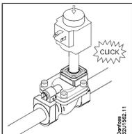
4. Mount the coil on the valve. The coil must **CLICK** in order to be positioned correctly.
