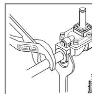
5. Use counterforce when tightening up pipe connections, i.e. use a spanner on both the valve body as well as on the pipe connector.
