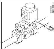
2. Use a screwdriver to lever the coil from the armature.
