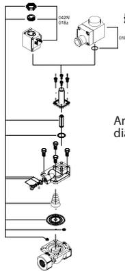
Armature, O-rings, spring, diaphragm
