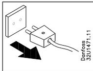
1. Before removing the coil, voltage must be disconnected, otherwise the coil will burn out.
