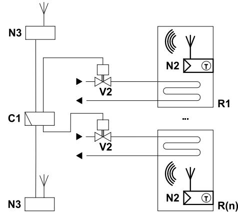
Room thermostat with floor heating and cooling with direct connection to the heat pump (floor cooling with RDZ200ZB only)
