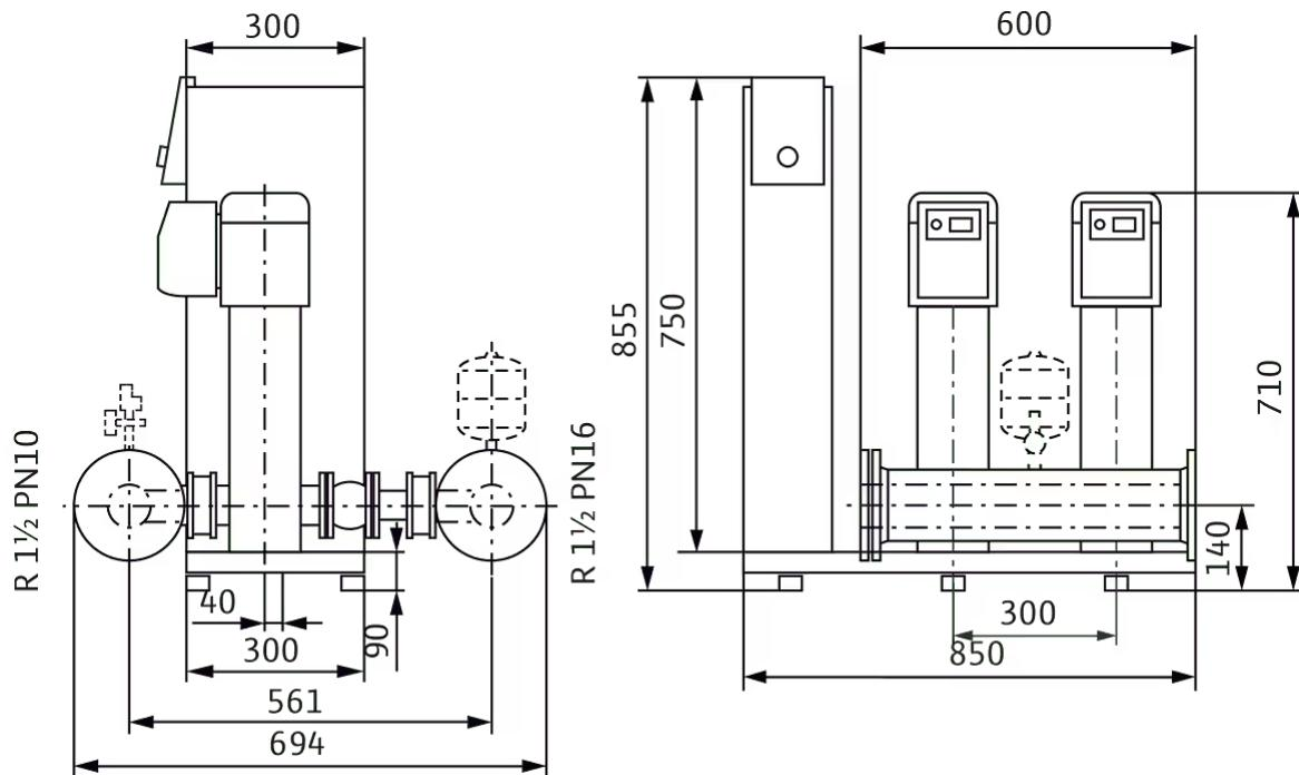
Sample systems are shown. Accessories (to be ordered separately): Optional WMS low-water cut-out switchgear kit; Installation surface: flat and horizontal Installation location: dry, well ventilated and frost-proof A working area of 1 m around the system is recommended in order to facilitate the maintenance process.
