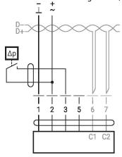
Switching contact requirements: The switching contact must be able to switch a current of 16 mA at 24 V accurately.
