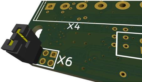
X6 Jumper Closed (Connected)
