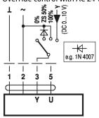
Control remotely 0...100% with positioner SG..
